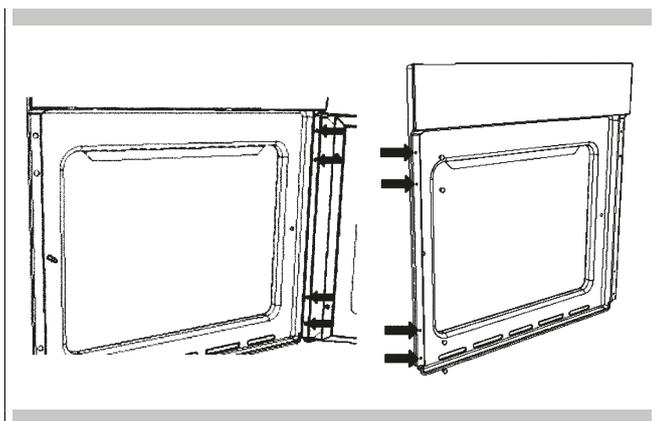
4. Remove the four plastic caps from the opposite side and unscrew the locking pin.
