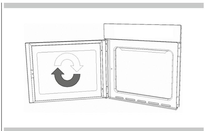
6. Secure the door in its new position using the 4 screws removed previously.
