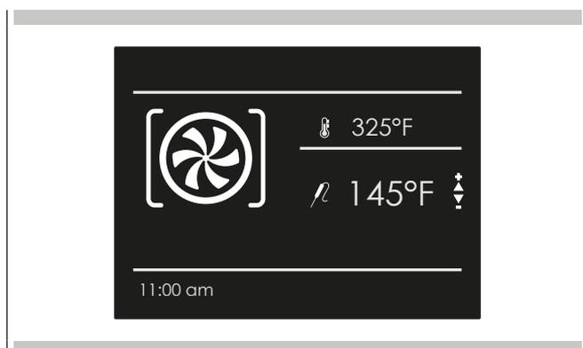
1. Set the required probe temperature by means of the arrows  $\Delta$   $\nabla$  and confirm with the  $\square$  key.
